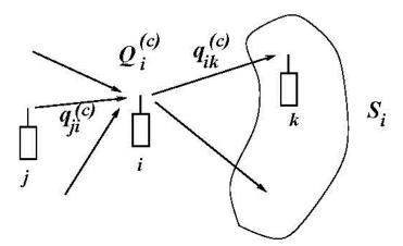
Fig. 1: The conservation of flow condition at node i for each commodity c requires that the sum of information generation rate and the total incoming flow must equal the total outgoing flow.
