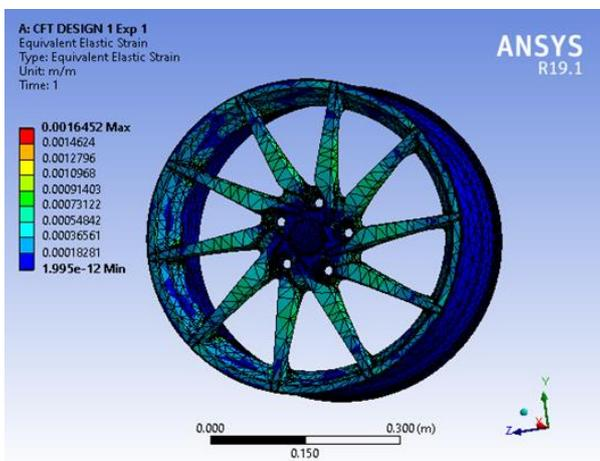
Fig. 2. Sample Strain Plot through FEA results
