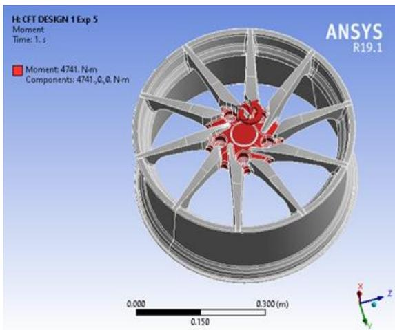
Fig. 1. Boundary conditions applied Sample
