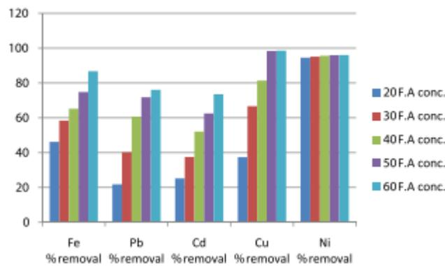
**Fig. 5 Efficiency of removal of a variety of heavy metals by the use of fly ash.**
