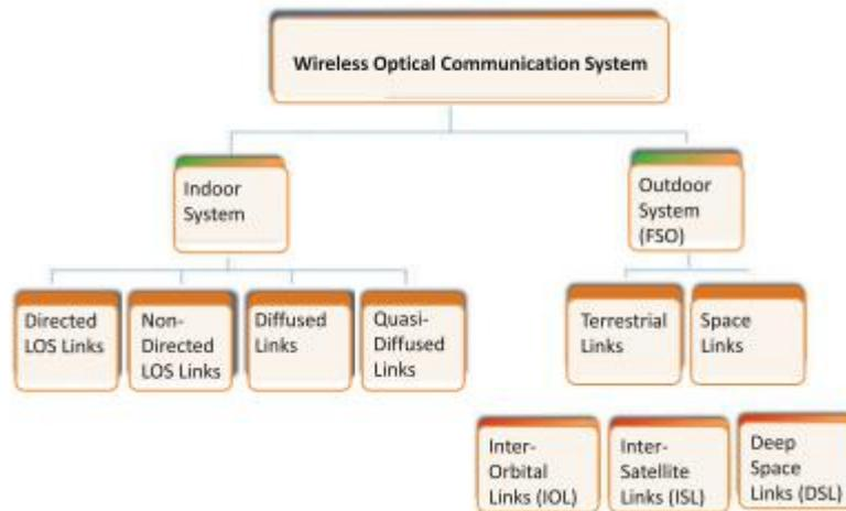
**Fig. 1. Classification of wireless optical communication systems**
