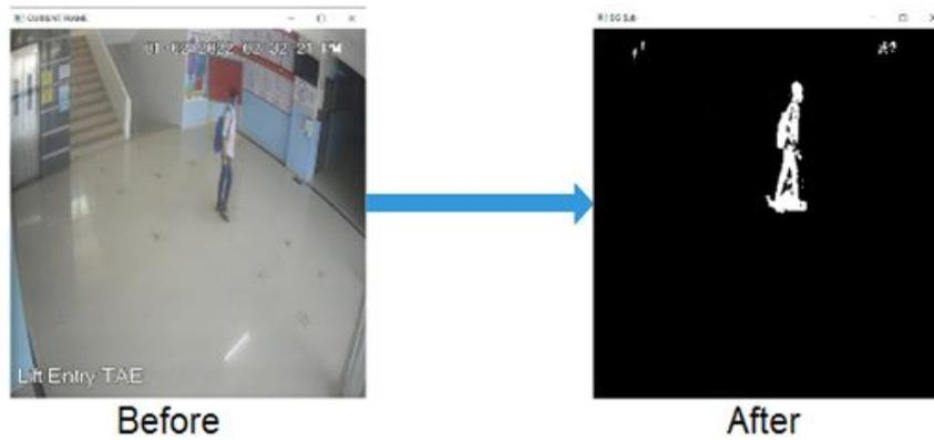
Fig.3. Background Subtraction using KNN
