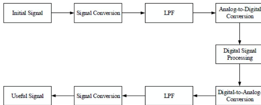
**Figure-1 : Digital Signal Processing flow**
